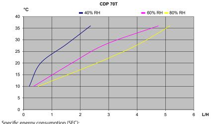
Specific energy consumption (SEC): 0,43 kWh/l at 28°C & 60% RH
