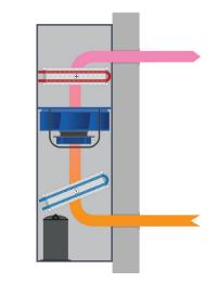
CDP 40T, 50T and 70T are designed for installation in an adjacent room and are supplied with a through-the-wall duct kit with supply and return air grills (accessory).
