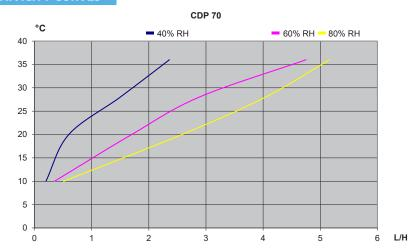
Specific energy consumption (SEC): 0,43 kWh/I at 28°C & 60% RH
