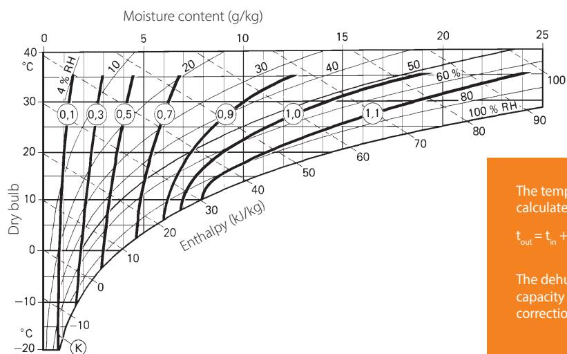
The temperature of the dry air at nominal air flows is calculated by:
