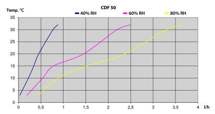
Specific energy consumption (SEC): 0,63 kWh/l at 20°C & 60% RH
